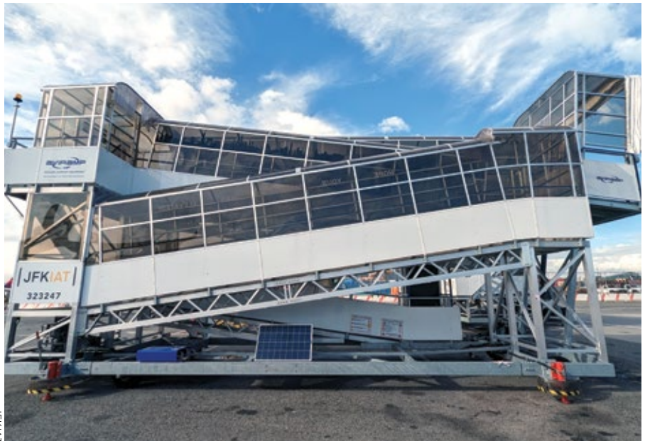
The JFKIAT Aviramp mobile jetbridge is a product designed by 'Aviramp' that allows all passengers to ascend/descend a ramp from the main aircraft door.
